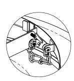
Use standard flat blade screwdriver to operate damper
